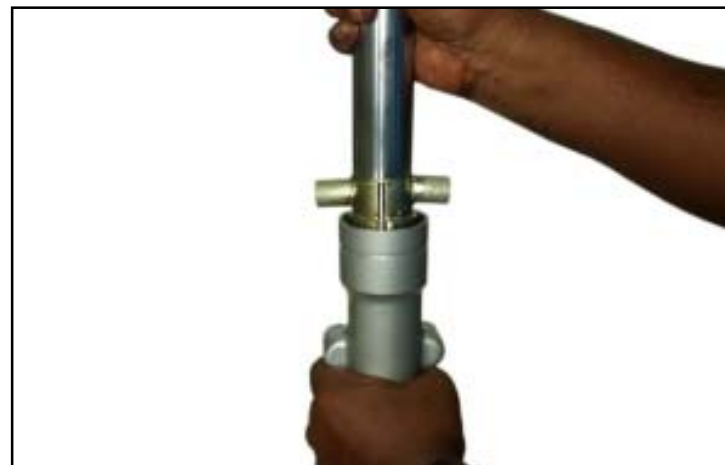
Application : Expander for oil seal while inserting main tube into bottom tube of front fork
