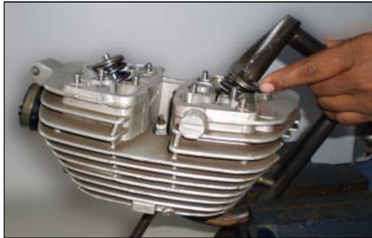
Application : To compress the valve spring for removal and fitting of valve.
