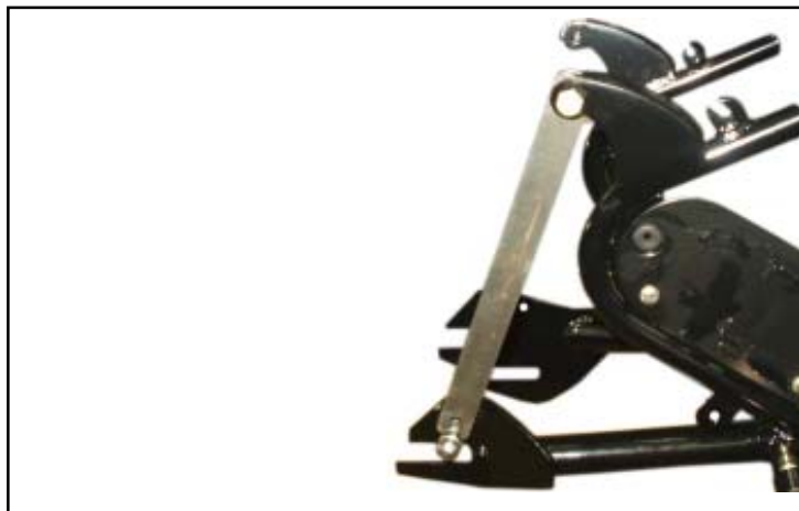
Application : Alignment of Swing Arm while tightening
