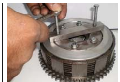
Application : To compress clutch springs while removing & refitting Clutch plates.
