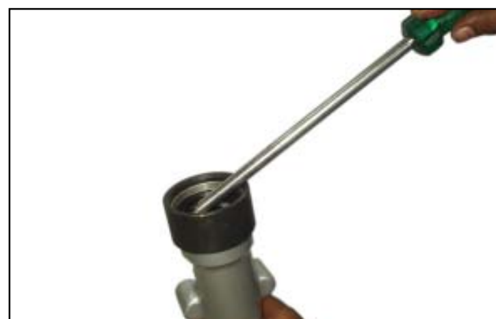
Application : Removal of oil seal in front fork bottom tube
