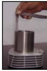
Piston ring end gap - Oil Ring
