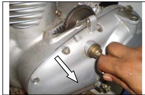
Application : To remove Crank case LH cover
