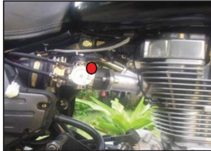
Assembled between air filter and inlet manifold
