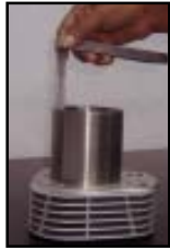
Piston ring end gap : compression
