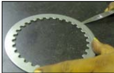
Clutch steel plate : Distortion
